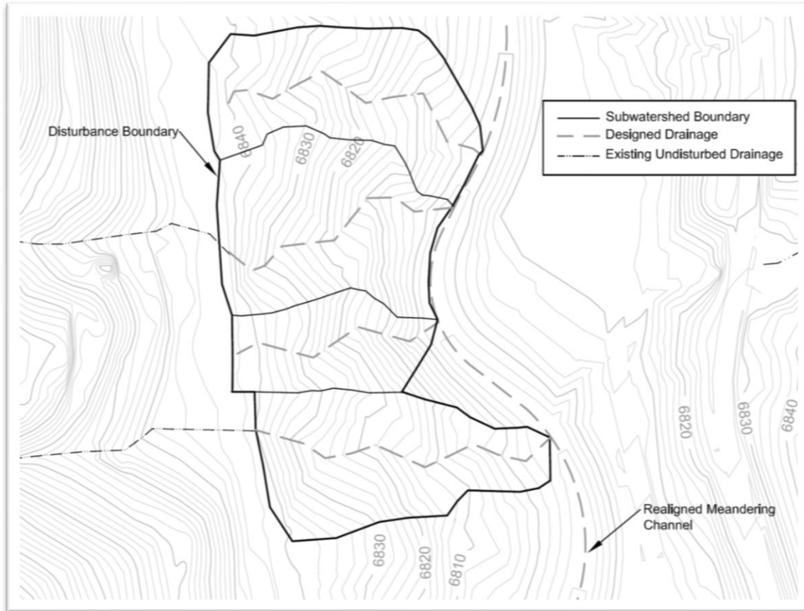
Figure 5. Design topography for a geomorphic landform at Swastika.
